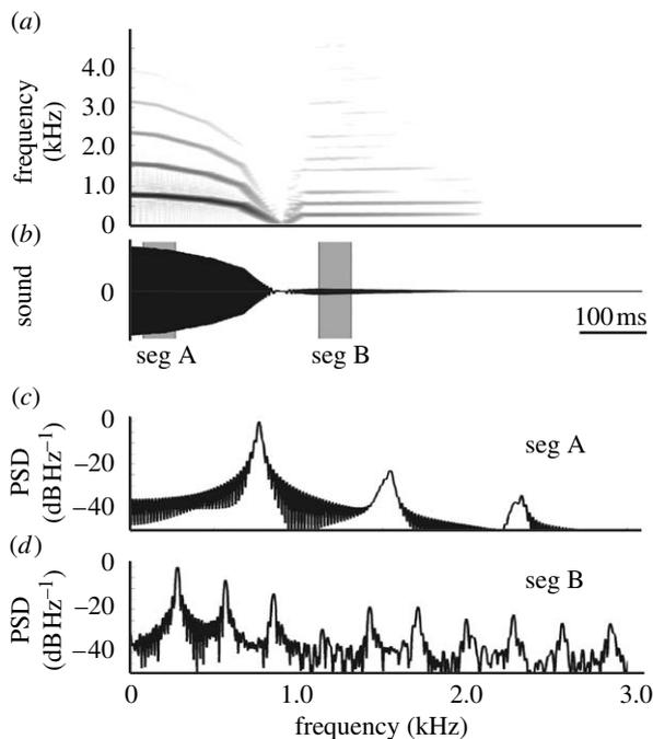
Figure 7. Simulation of the asymmetry expiration/inspiration. (a) Spectrogram and (b) oscillogram of expiratory and inspiratory note simulation. (c) Power spectral density (PSD) estimations of segment A (seg A) during expiration and (d) segment B (seg B) during inspiration. Segments are taken from (b) as indicated.
